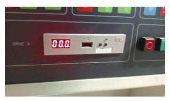
Flash drive can now be used to save programs from PC to Charmilles. This will follow the same procedure as before. Verify that the Emulator reads 000, with flash drive inserted, can copy down files from the A:\ drive just like it was a regular floppy.
